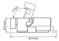
2. Front lock structure with tactile feedback
